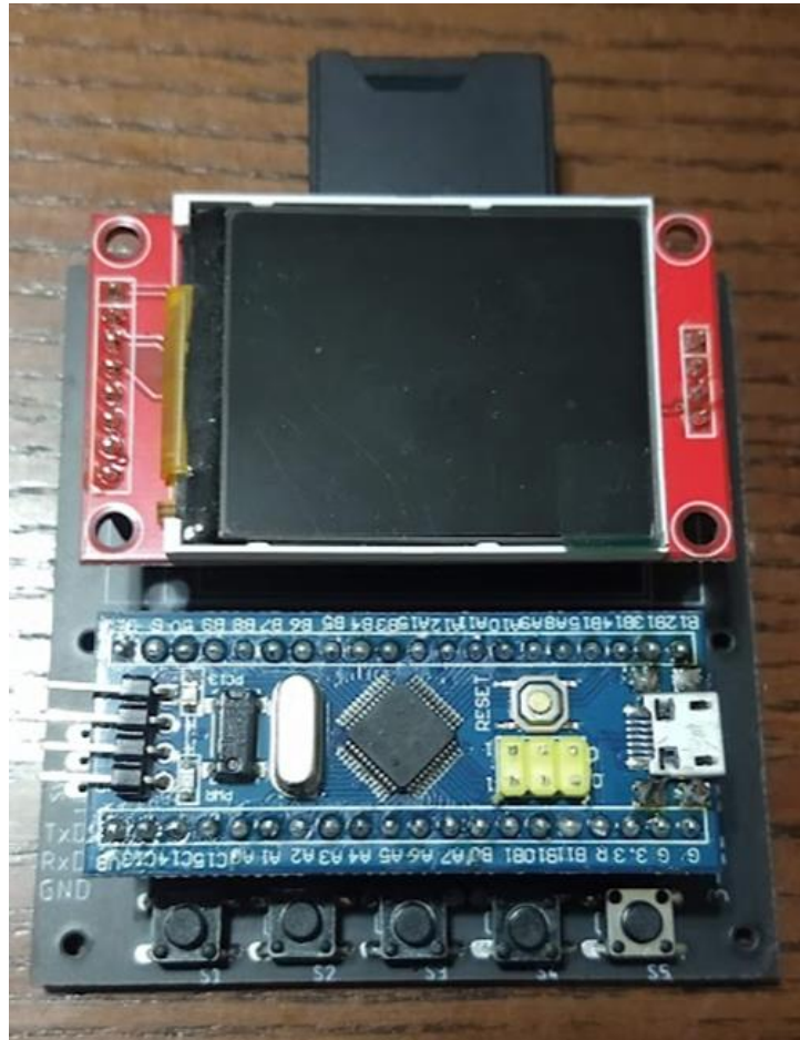
Figure 8: Fully Assembled PCB with Boot 0/1 Headers Removed Note: To fit in the provided 3D case, please remove Boot 0/1 Headers
