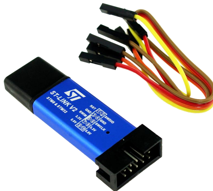
Figure 3: ST-LINK V2 - programming the Bluepill
